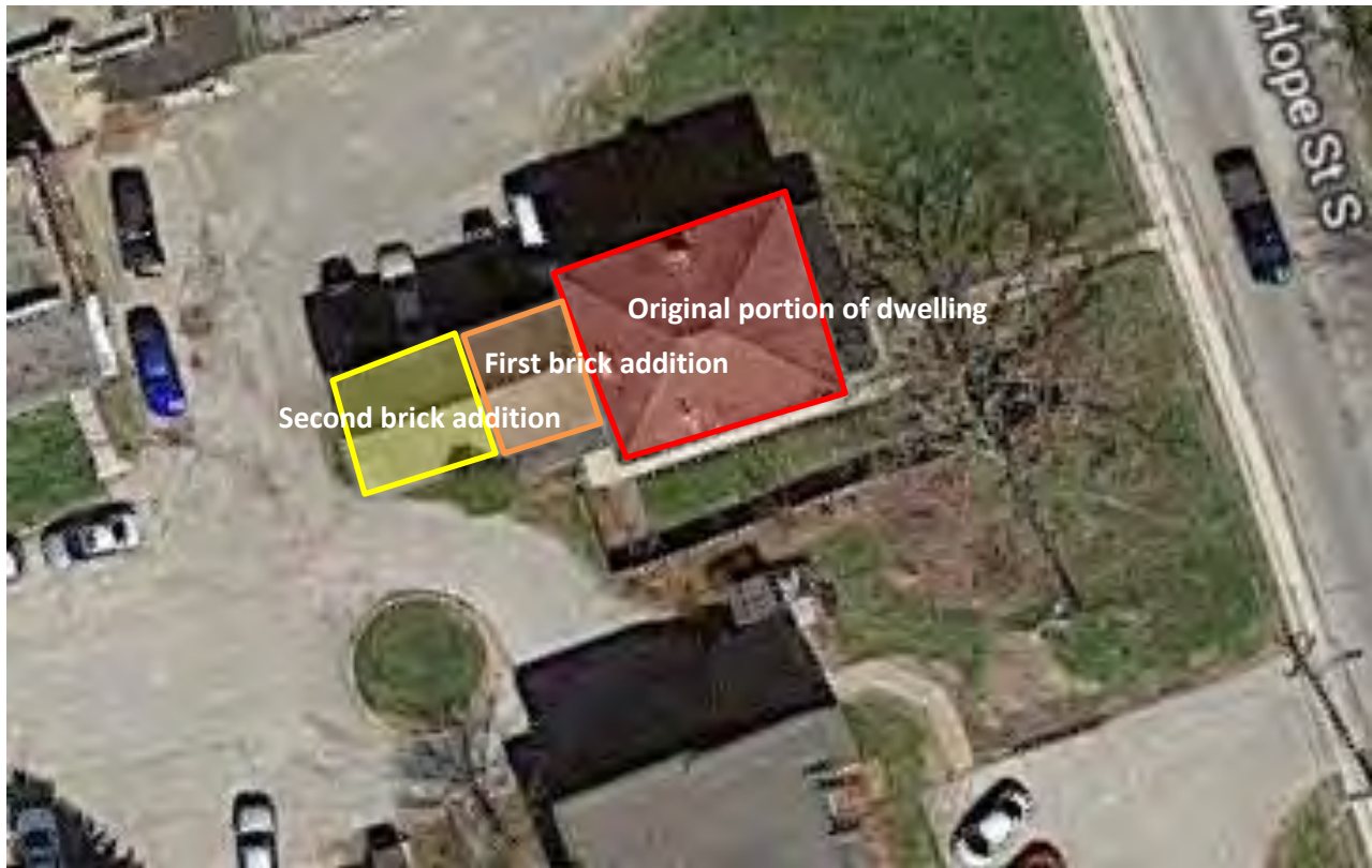
Figure 42: Aerial photo of context and study area, detail view of 36-38 Hope Street. (Source: Northumberland County Interactive Map, 2018)
